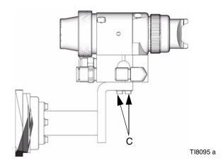
Fig. 6: Stationary Support Mount
